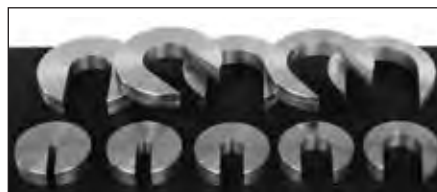
Auxiliary tools for dismantling of inner rings and delicate components.
